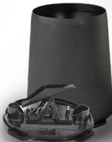
The IRG02, is a tipping-bucket rain gage. It measures rainfall in 0.01 in. increments. The IRG02 funnels precipitation into a bucket mechanism that tips when filled to its calibrated level. A magnet attached to the tipping mechanism actuates a switch as the bucket tips. The momentary switch closure is counted by the pulse-counting circuitry of our data loggers.
